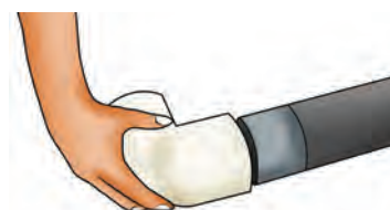
Fig.1.12: Assemble the edges when the cement solvent is wet
