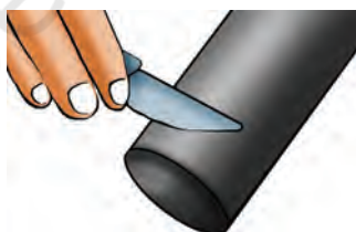
Fig.1.11: Apply the solvent on both the edges
